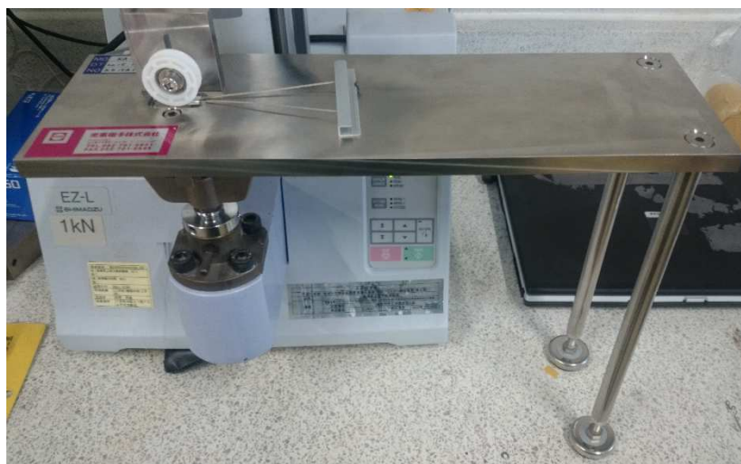
Fig.26 A jig for the measurement of coefficient of friction.
