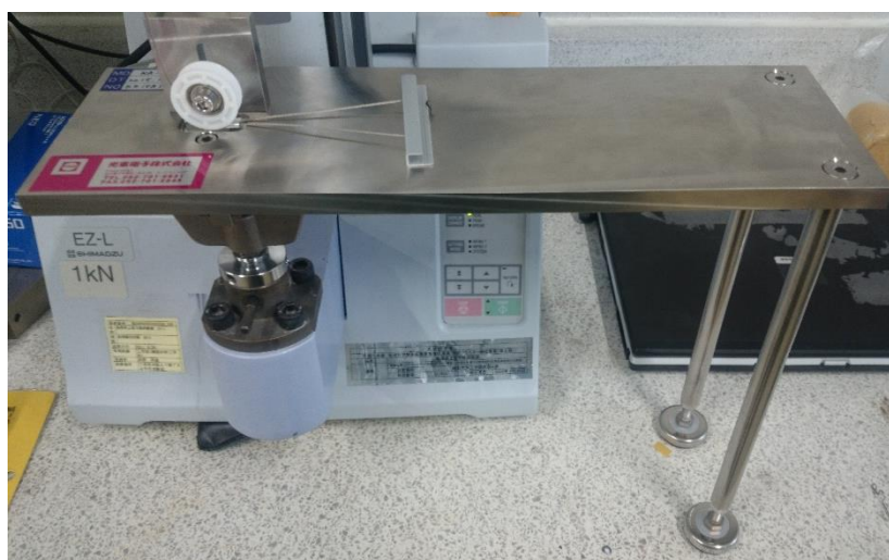
Figure 5-4 A jig for the measurement of coefficient of friction.
