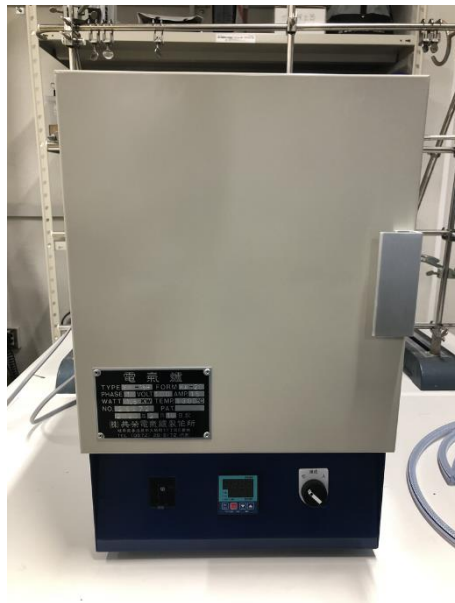
Fig. 2-8 Appearance of Electric furnace (YK-15B).
