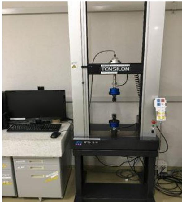
**Fig. 2.2 Appearance of Universal testing machine (RTG-1310).**
