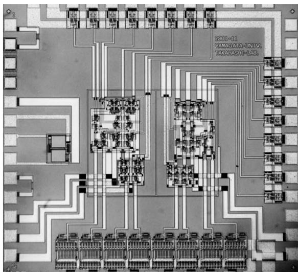
**Fig. 7** Photomicrograph of 1 bit adder/subtractor chip.
