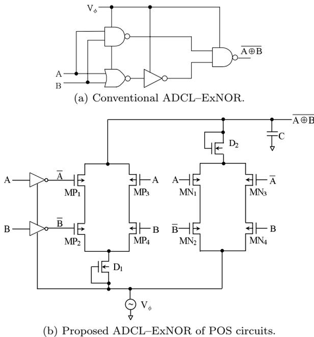
Fig. 5 ExNOR gates for ADCL circuit technology.
