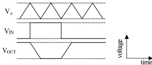
Fig. 3 Output waveform of ADCL-NOT in adiabatic mode.
