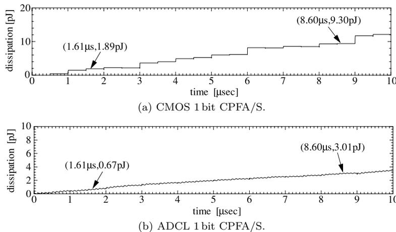
Fig. 6 Energy dissipation for PSPICE simulation.
