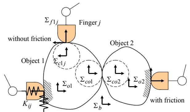
Figure 1: Two objects grasped by a multi-fingered hand.
