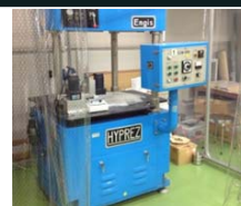
Commercially available single-sided polisher (Engis Japan : HYPREZ-610)
