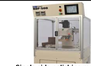
Single side polishing machine (Fujikoshi Machinery Corp.: RDP-500)
