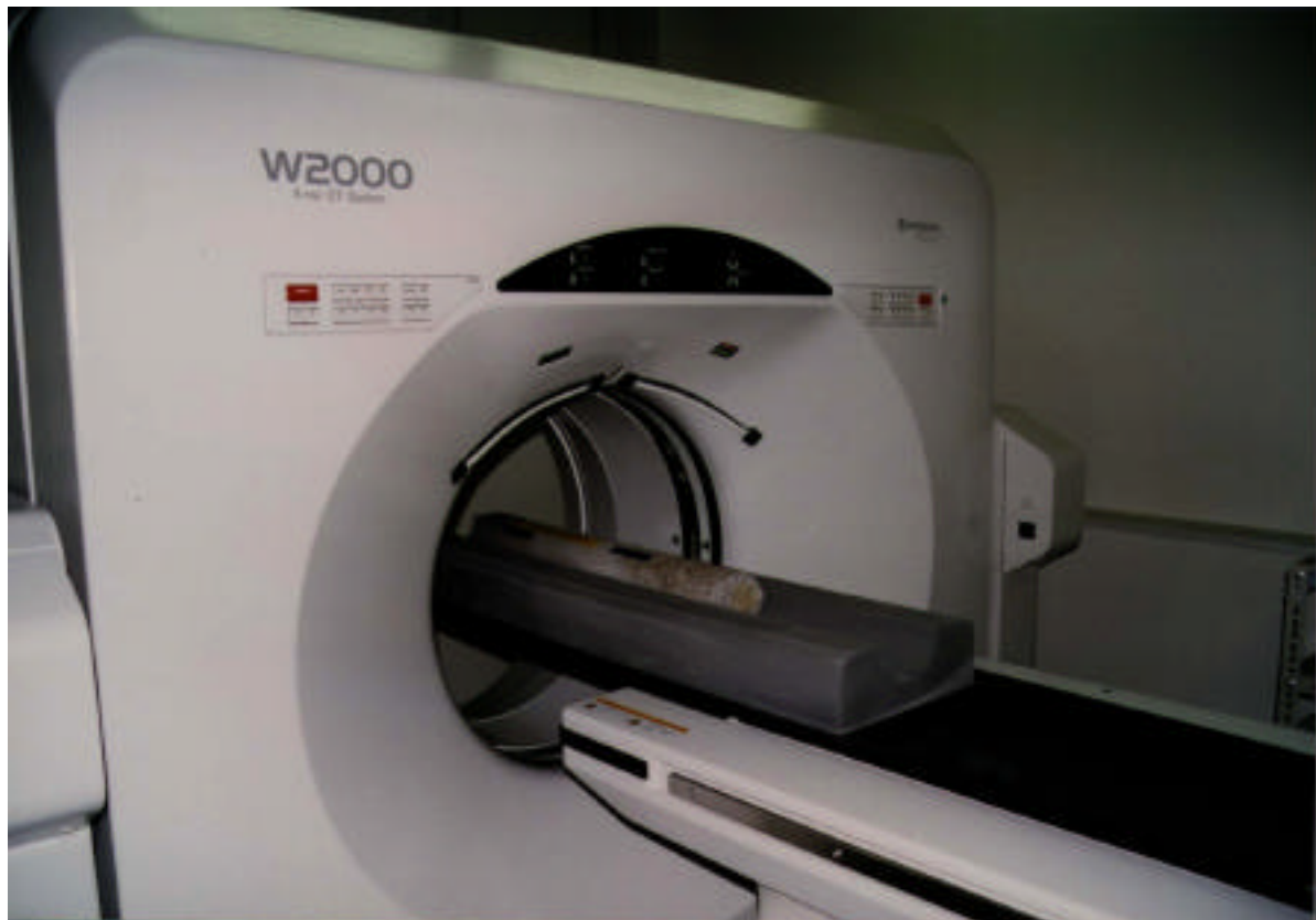
Fig.1 X-ray CT scanner used in this study. The diameter of the core is 10.15cm.
