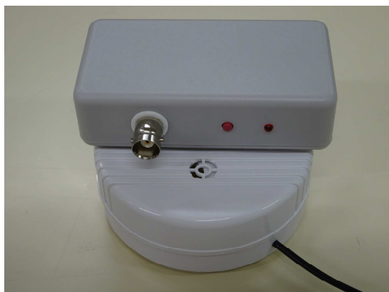
Fig.10: Connection between water leak sensor unit and WAN-WAN basic module
