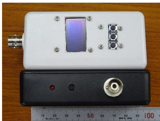
Fig.9: Connection between thermocouple unit and WAN-WAN basic module
