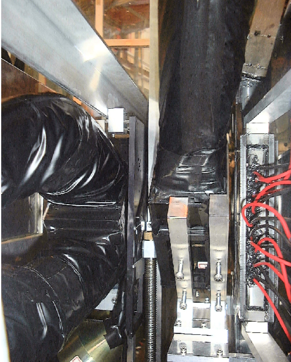
Figure 2.5: Photograph of the target region seen from the side. The beam entered from the left side of the picture. The two black blocks are scintillating fiber block detectors.
