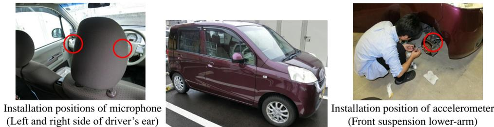
Fig. 2 Photographs of test vehicle.
