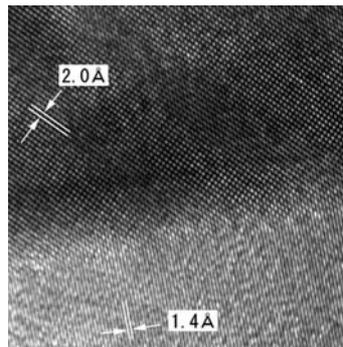
金結晶薄膜 (直接倍率 x1,000,000)
