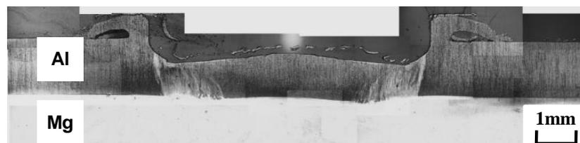
Fig.2 Macroscopic appearance in cross section of Al/Mg FSSW joint.
