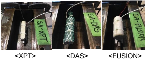
Picture 2. Sacrificial anodes that are used
